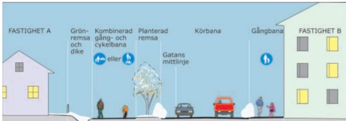
The diagram illustrates a street section with various property boundaries (Fastighet A and Fastighet B) and shared areas. It shows a house, a green embankment, a combined pedestrian and cycling path, a planted curb, a carriageway, a sidewalk, and a crosswalk. Responsibility for different tasks is assigned to the property owners or the municipality.
